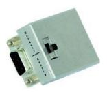
The D-ADAPT-MPC4 Service Adapter is connected via the 6-pole service interface to a D-ADAPT-MPC4 ETH / WLAN Enterprise network adapter and enables so the connection of a PC via RS232 interface (9-pole D-SUB socket) to configure the network adapter.
