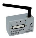
D-ADAPT-MPC4 WLAN enables the DBL battery charger series with MPC4 controller board to be connected to a Wireless LAN network (IEEE 802.11b/802.11g) for data transmission with max. 11 mbps. The adapter supports among others WEP/WPA/WPA2 and RADIUS server authentication / PSK (pre-shared keys).
